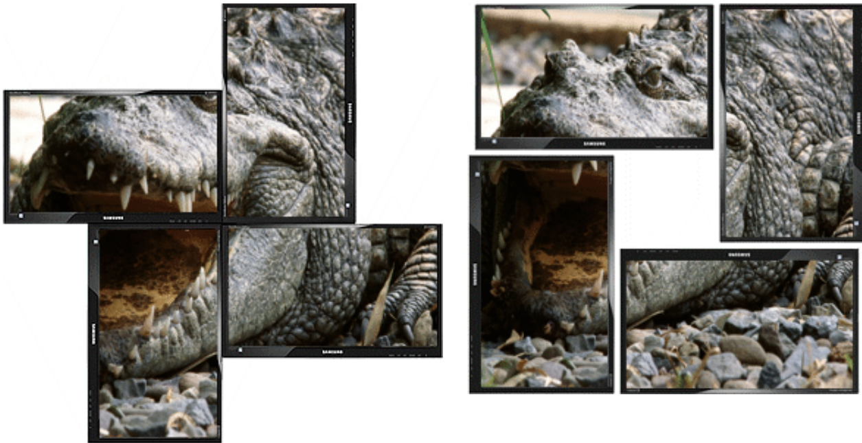
Crop the input signal into x4 and display x2 quarters landscape and x2 quarters portrait.
